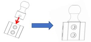
a. Align the hitch ball hole with the center of the bracket hole
